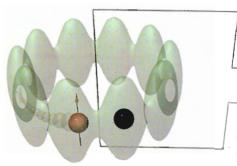
A proposed quantum motor that may one day do work would be made up of a carrier atom (brown with an arrow) and a starter atom (blue) trapped in a ring.
