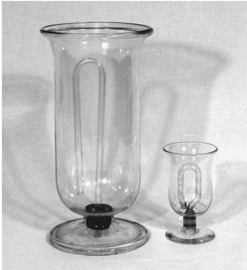
Dribble Glasses. More properly, these two glasses in the collection of Union College in Schenectady, New York, are examples of Tantalus cup or the automatic siphon. When the water level reaches the bend in the internal glass tube, the siphon starts and the glass empties itself of water. (Photograph and Notes by Thomas B. Greenslade, Jr., Kenyon College)
