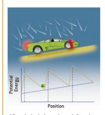
When the brake is on, the car is forced down into the notch of the sawtooth. It is unlikely that a hailstone would push the car out of this locked position. (If one did, the car would actually tend to move backward—that is, the path of least resistance for the ratchet.)
