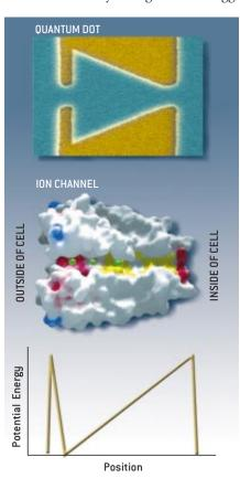
TWO RATCHETS differ in detail but may work in basically the same way. The micron-size triangular quantum dot, etched onto a silicon wafer, is a diode-a device that turns alternating current into direct current. The ion channel—a protein molecule shown here as a cutaway surface—is a biological version of a diode, a hundredth the size of the dot. The potential energy profile is thought to be the same for both devices.
