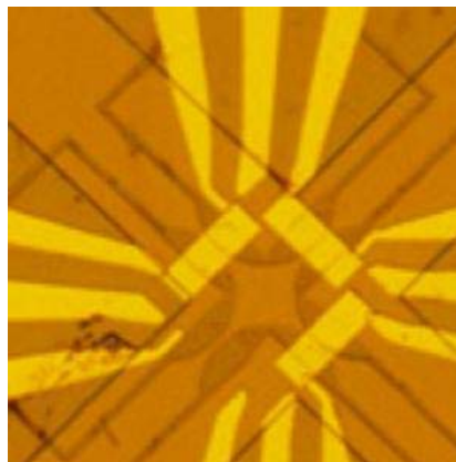
Circuit with quantum point contacts. (Credit: Image courtesy of Technische Universitaet Muenchen)
