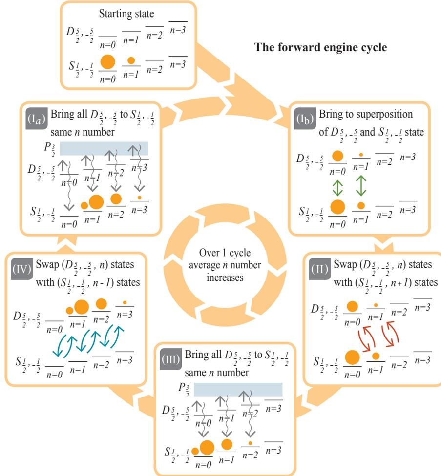
Supplementary Figure 1: **Pictorial description of the forward engine cycle.** The initialized starting state is shown, followed by strokes (I<sub>b</sub>) through (IV), and finally back to (I<sub>a</sub>). The diameter of the orange circles represents the probability of the ion being in the corresponding state.
