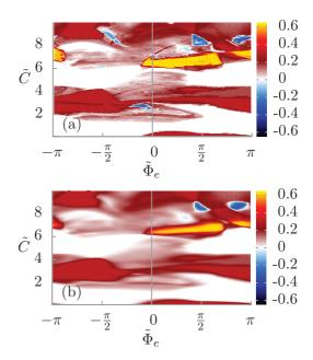
FIG. 11. (Color online) Voltage across the the rocked SQUID in the parameter plane  $\{\Phi_e, \tilde{C}\}$ . Upper panel: the deterministic case D=0. Lower panel: influence of temperature  $D=10^{-3}$ . The dc current F=0.1. The remaining parameters are a=2.4,  $\omega=0.31$ , j=1/2.
