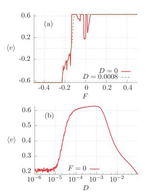
FIG. 6. (Color online) Constructive influence of thermal noise on the ratchet effect. (a) The current-voltage characteristics is presented in the deterministic limit (D=0, solid red line) and the noise-driven case (D=0.0008, dashed green line) case. (b) The dependence of the average voltage  $\langle v \rangle$  on the thermal noise intensity D. The remaining parameters are  $a=2.3, \omega=0.63, \tilde{C}=1.98, j=1/2,$  and  $\tilde{\Phi}_e=\pi/2$ .
