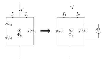
FIG. 1. The asymmetric SQUID composed of three Josephson junctions and the equivalent circuit composed of two junctions, where the Josephson phase difference is  $\varphi_1 = \varphi_u + \varphi_d$ . The physical quantity of interest is the long-time average voltage V across the SQUID which is expressed by the relation  $V = \hbar \langle \dot{\varphi}_1 \rangle / 2e = \hbar \langle \dot{\varphi}_2 \rangle / 2e$ ; see Eq. (A1) in the Appendix.
