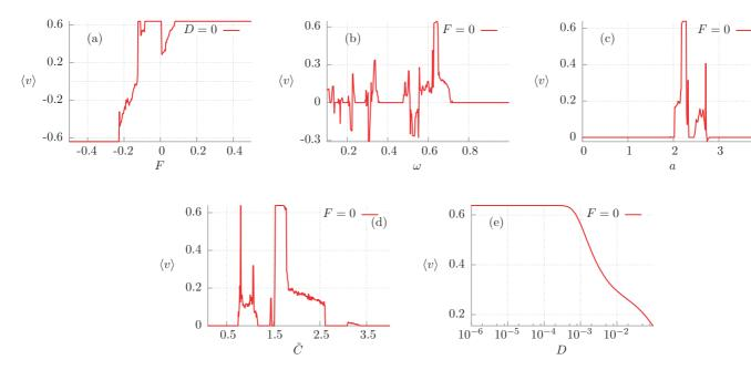
FIG. 9. (Color online) Optimal regime for the occurrence of the ratchet transport. The dependence of the average voltage  $\langle v \rangle$  on the static dc bias F, the angular frequency  $\omega$ , amplitude a, capacitance  $\tilde{C}$ , and thermal noise intensity D is presented in (a)–(e). The chosen parameters are D=0, F=0, a=2.25,  $\omega=0.638$ ,  $\tilde{C}=1.65$ , j=1/2, and  $\tilde{\Phi}_e=\pi/2$ .
