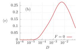
FIG. 8. (Color online) Noise-induced ratchet effect. (a) shows the current-voltage characteristic in this regime. (b) depicts the dependence of the average voltage  $\langle v \rangle$  on the thermal noise intensity D in the absence of a bias F=0. Other parameters are a=1.8,  $\omega=0.56$ ,  $\tilde{C}=1$ , j=1/2, and  $\tilde{\Phi}_e=\pi/2$ .
