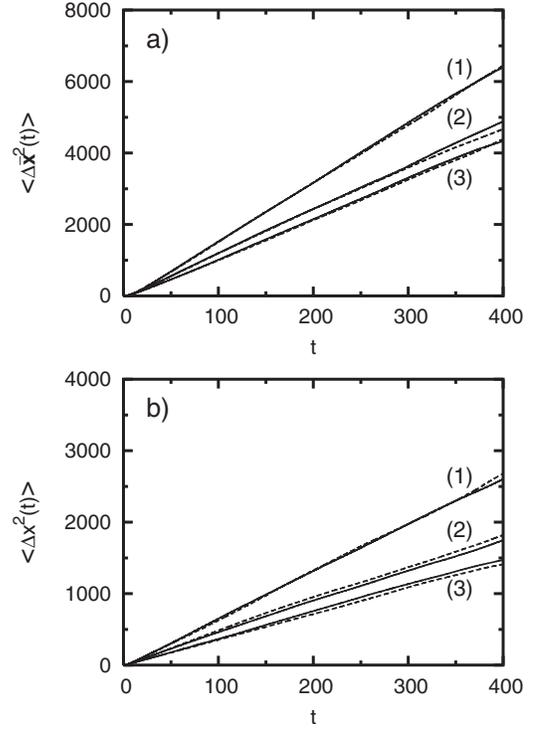
FIG. 2. Plots of MSD as a function of time obtained from the MD simulations for various values of  $q$  and  $\alpha$  (a) for the slit pore system and (b) for the cylindrical pore system at  $\rho=0.01$ . The MSD using the MP wall is plotted with solid lines and the MSD using the Knudsen-Smoluchowski wall is plotted with dashed lines. (1)  $q=0.3$ ,  $\alpha=0.6$ ; (2)  $q=0.4$ ,  $\alpha=0.8$ ; and (3)  $q=0.5$ ,  $\alpha=1$ .
