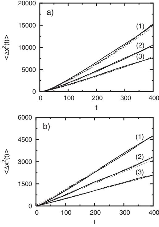
FIG. 1. Plots of MSD as a function of time obtained from the MD simulations for various values of  $q$  and  $\alpha$  (a) for the slit pore system and (b) for the cylindrical pore system at  $\rho=0.0001$ . The MSD using the MP wall is plotted with solid lines and the MSD using the Knudsen-Smoluchowski wall is plotted with dashed lines. The analytical results of MSD are displayed with dotted lines. (1)  $q=0.3$ ,  $\alpha=0.6$ ; (2)  $q=0.4$ ,  $\alpha=0.8$ ; and (3)  $q=0.5$ ,  $\alpha=1$ .
