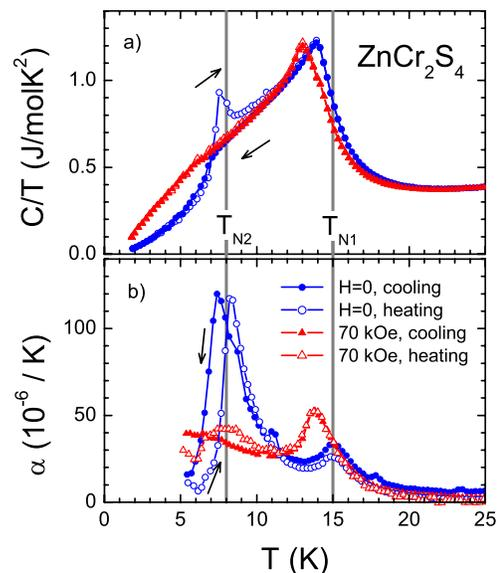
FIG. 2 (color online). (a) Heat capacity of  $\text{ZnCr}_2\text{S}_4$  plotted as  $C/T$  vs  $T$  measured on cooling (closed symbols) and heating (open symbols) for 0 and 70 kOe. (b) Temperature dependence of the thermal-expansion coefficient at different magnetic fields. Vertical lines: the phase transitions  $T_{N1}$  and  $T_{N2}$  in zero field.
