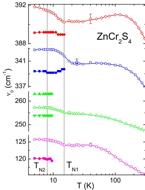
FIG. 4 (color online). Temperature dependence of the eigenfrequencies of the all phonon modes on a semilogarithmic plot. Open symbols: fundamental modes; closed symbols: the new modes below  $T_{N1}$  and  $T_{N2}$ .
