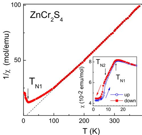
FIG. 1 (color online). Inverse susceptibility vs temperature as measured in  $\text{ZnCr}_2\text{S}_4$  at 10 kOe. The dashed line indicates a CW behavior. Inset: Low-temperature susceptibility for heating (up) and cooling (down) cycles.
