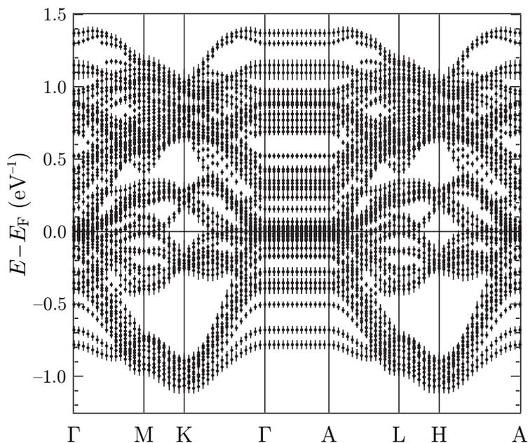
**Figure 5.** Weighted electronic bands for a prototypical V atom in a  $V_2O_3$  thin film, located  $\approx 28 \text{ \AA}$  beneath the surface. The length of the bars shown for each state is proportional to the contributions of this atom. States with a contribution below a certain threshold are omitted for clarity.
