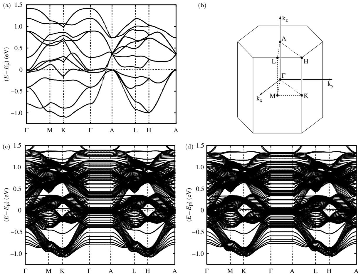
**Figure 4.** Electronic band structure of bulk  $V_2O_3$  (top left), for high symmetry lines in the first Brillouin zone of the hexagonal lattice (top right), compared to a  $V_2O_3$  thin film with bulk lattice constants (bottom left) and with a 1% elongated  $c$  lattice constant (bottom right).
