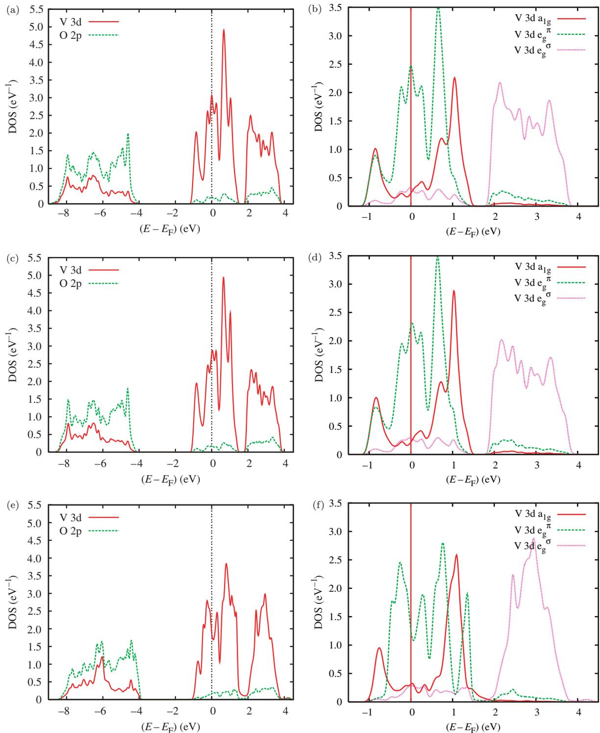
**Figure 3.** Partial V 3d and O 2p DOS (left) as well as V 3d symmetry components (right) for a  $\text{VO}_6$  octahedron in bulk  $\text{V}_2\text{O}_3$  (top row), separated by  $\approx 28 \text{ \AA}$  from the surface of a  $\text{V}_2\text{O}_3$  thin film (center row), and at the surface of a  $\text{V}_2\text{O}_3$  thin film (bottom row). All DOS curves are per formula unit.
