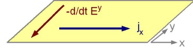
FIG. 2. (Color online) Setup for a transverse spin current driven by a time-dependent electric field in the presence of spin-orbit coupling.
